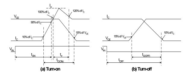
Figure 4. Switching Time Definition
