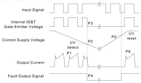
P1: Normal operation: IGBT ON and conducting current.
