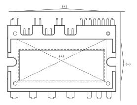
Figure 6. Flatness Measurement Position
