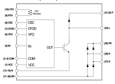
Figure 3. Internal Block Diagram
